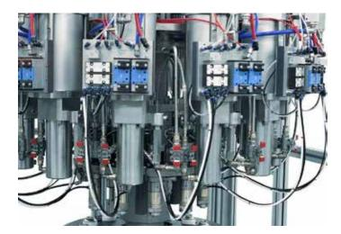
Through-The-Valve (TTV) Air-Powered Propellant Filler
