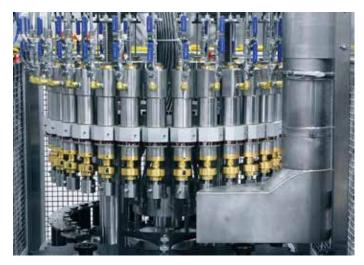
Through-The-Valve (TTV) Propellant Filler
