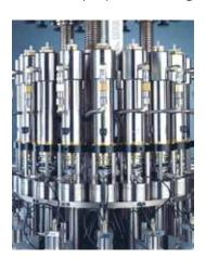
Positive displacement propellent powered metering cylinders ensure precision fills. Cylinders have a capacity of 550cc and are propellant powered eliminating heat buildup typical with air powered cylinders when using compressed gasses such as CO2 and N2O. KP-Aerofill AG-275 offers 249 degrees of rotation for propellant filling and 226 degrees of rotation for shaking.
