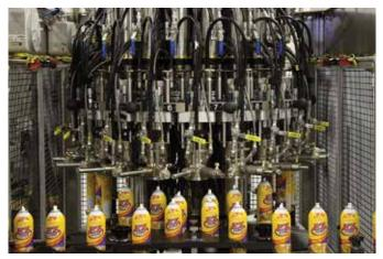
Rotary Under-The-Cup (UTC) Propellant Filler
